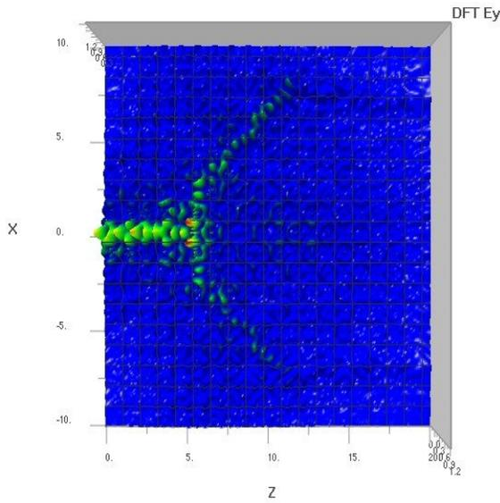
Fig. 4 (b) Electric Field Distribution of Y splitter profile
