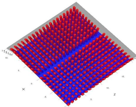
Fig. 3(a) Refractive Index Profile with Line Defect Waveguide
