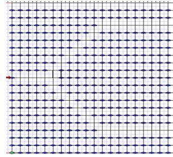
Fig. 5 (a) Crystal lattice layout of elliptical Y splitter
